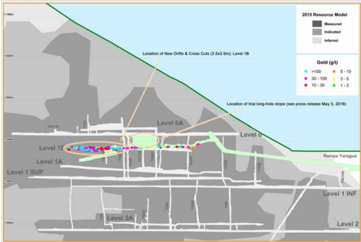
Figure 3 – Long section of the Yaraguá Mine showing the locations of the new underground development relative to the trial mining stope announced on May 3, 2016.
